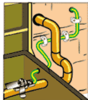
Detail showing main bonding conductor: BS 951 clamp. 'SAFETY ELECTRICAL CONNECTION - DO NOT REMOVE' label and holes in the gas meter box and the wall.
